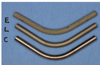
Figure 10. Machined Ti6Al4V vs DMLS and EB Ti6Al4V after four point bending static test
